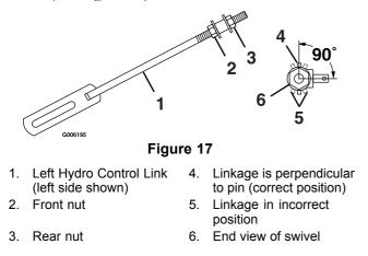
After adjusting the left hydro control linkage, move the speed control lever to the mid-speed position and then back to the neutral position. Recheck the left drive wheel rotation to see if further adjustment is necessary - be sure the speed control lever is in the neutral position.
